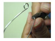
4.) pinch the end of the wire with the edge of flat nose plier, & turn a 90° angle.
